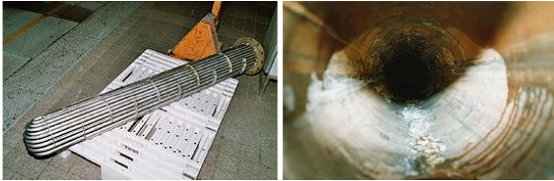
Heat exchange core (left) / inside of the heat exchanger housing (right)
